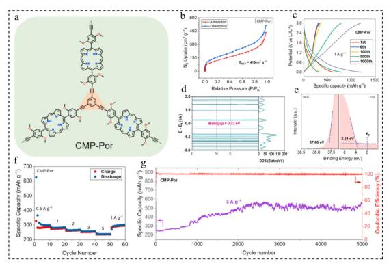
Fig. 12 (a) Structure of CMP-Por. (b) BET test for CMP-Por. (c) GCD profiles at 1 A g<sup>-1</sup>. (d) Density of states of CMP-Por. (e) Ultraviolet photoelectron spectroscopy of CMP-Por. (f) Rate capability. (g) Long-term cycle life at  $\overline{3}$  A  $g^{-1.103}$  Copyright 2022, Elsevier.
