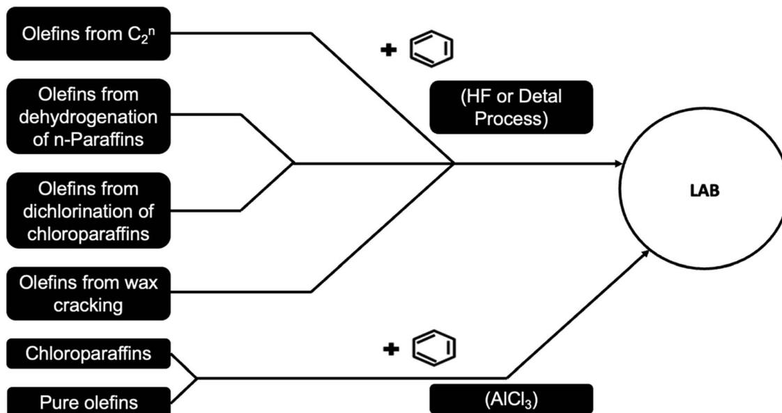
Fig. 5 The most common LAB production methods (adapted from Shokri and Karimi).<sup>3</sup>
