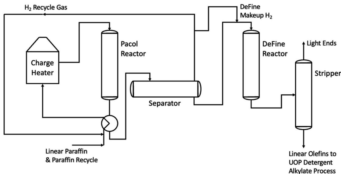
Fig. 6 UOP Pacol dehydrogenation process (adapted from Bhasin *et al.*).<sup>4</sup>
