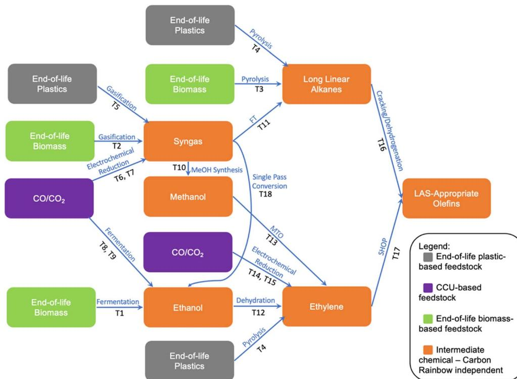
Fig. 3 Defossilised routes to LAS-appropriate olefins (edited from Platt and Styring).<sup>2</sup> Number labels have been added for future reference.
