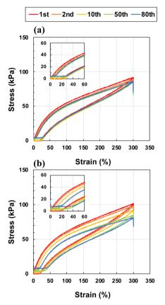
Fig. 5 Cyclic stress–strain curves at 300% strain at a tensile rate of  $10 \text{ cm min}^{-1}$  for the ion gels with cross-linker contents of (a) 0.01 mol% and (b) 0 mol% at the same initiator content of 0.02 mol%. Each cycle was separated by a waiting time of 600 s. The inset shows magnified images.
