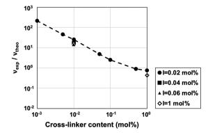
Fig. 3 Relationship between the cross-linker content in the pre-gel solution and the ratio of experimental to theoretical cross-linking densities  $(\nu_{\rm exp}/\nu_{\rm theo})$  of the ion gels.
