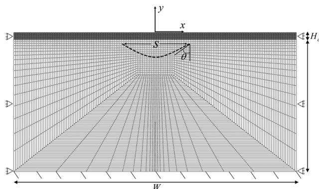
Fig. 2 Finite element mesh and boundary conditions. The full domain of  $W \times H$  is split into the cortical layer with thickness  $H_c$  and the subcortical layer with thickness  $H_s$ . The horizontal span of the axonal tract,  $s$ , and the angle of the parabola at the right intersection,  $\theta$ , are also shown.
