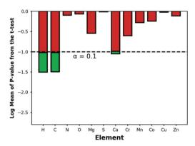
Fig. 9 Statistical significance for comparison of elemental compositions between the top-14 MOFs and the entire database based on the p-values derived from the t-test. The dashed line represents our chosen critical value for the one-sided t-test. Bars that fall below this threshold indicate elements that are statistically significantly more abundant in the top-performing MOFs. Ca is a metal that appears significantly more frequently in the top-14 MOFs than in the full database.
