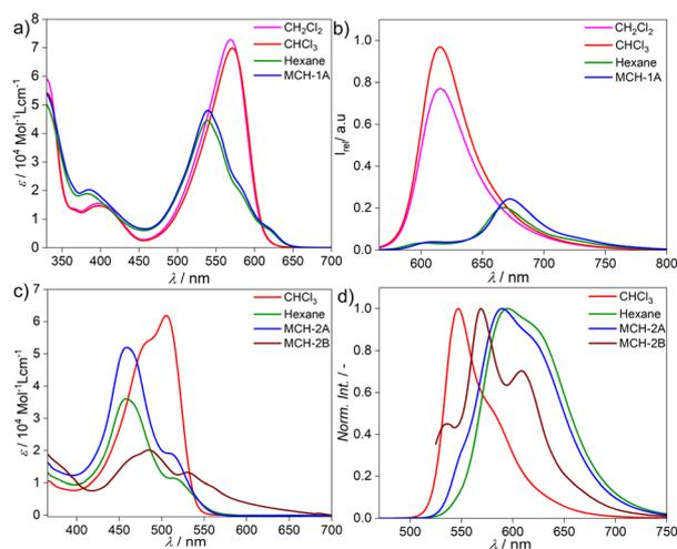
Fig. 1 Solvent-dependent absorption studies of: (a) compound **1**, (c) compound **2** and solvent-dependent fluorescence studies of: (b) compound **1**,  $\lambda_{\text{exc}} = 510$  nm and (d) compound **2**,  $\lambda_{\text{exc}} = 470$  nm at 298 K,  $c = 2 \times 10^{-5}$  M.
