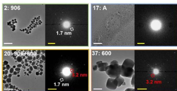
Fig. 11 Zoom-ins with enlarged diffraction patterns for selected samples from an array. The observed phases are denoted as A (amorphous product), 906 (NU-906), or 600 (NU-600). White scale bars = 2  $\mu\text{m}$ . Yellow scale bars = 0.5  $\text{nm}^{-1}$ . Reprinted (adapted) with permission from Gong *et al.*<sup>255</sup> Copyright 2022 American Chemical Society.
