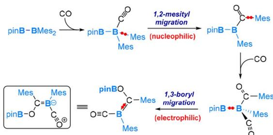
Scheme 4 Mechanism of the reaction of pinB-BMes<sub>2</sub> with CO.
