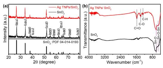
Fig. 1 (a) XRD patterns and (b) FTIR spectra of SnO<sub>2</sub> and Ag TNPs/SnO<sub>2</sub>
