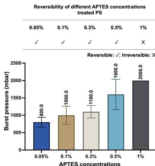
Fig. 2 Reversibility and burst pressure of devices based on different concentrations of APTES-treated PS. The burst resistance of the devices increased with higher APTES concentrations ( $n = 6$ ).
