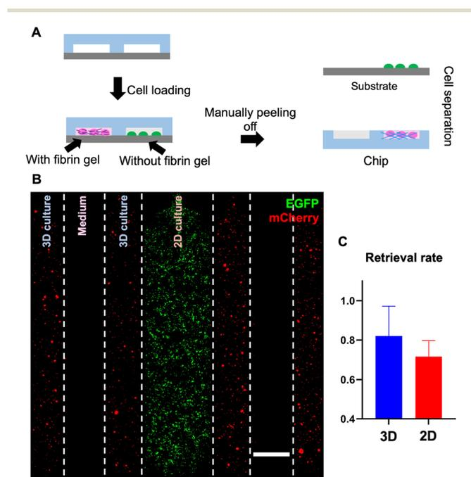
**Fig. 7** A: Workflow for assessing the retrieval rate from 3D and 2D cell culture channels of the reversible device; B: two types of cells compartmentalized with different culture methods within the multi-channel device (bar = 1 mm); C: above 70% retrieval rate of 3D and 2D cell culture ( $n = 3$ ).
