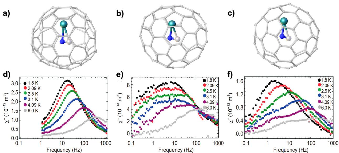
Fig. 5 Molecular structures of  $\text{TbCN@C}_2(5)\text{-C}_{82}$  (a),  $\text{TbCN@C}_s(6)\text{-C}_{82}$  (b) and  $\text{TbCN@C}_{2v}(9)\text{-C}_{82}$  (c). Out-of-phase AC magnetic susceptibility of  $\text{TbCN@C}_2(5)\text{-C}_{82}$  (d),  $\text{TbCN@C}_s(6)\text{-C}_{82}$  (e) and  $\text{TbCN@C}_{2v}(9)\text{-C}_{82}$  (f) at 1.8–6 K. Reproduced from ref. 100.
