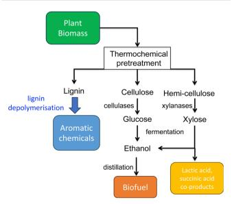
Fig. 1 Schematic representation of lignocellulosic biorefinery.
