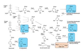
Fig. 13 Production of bioproducts from lignin using engineered recombinant bacterial strains. Aromatic products shown in blue, non-aromatic products shown in brown
