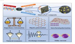
Fabrication of iron manganese metal-organic framework derived magnetic MnFe<sub>2</sub>O<sub>4</sub>/C composites for broadband and highly efficient electromagnetic wave absorption
