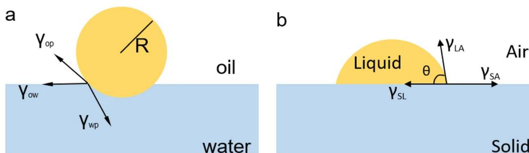
Fig. 1 (a) A schematic illustration of the interfacially adsorbed NP, where  $R$  is the radius of NP. (b) Schematic illustration of a sessile droplet on a solid surface, with the relationship between the CA and surface tension  $\gamma$ . Reproduced with permission.<sup>22</sup> Copyright © 2019 Wiley-VCH GmbH.
