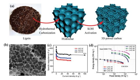
Fig. 3 (a) Schematic of the synthesis of LHC samples. (b) SEM image of the LHC-3K. (c) Rate performance of the LHC-based electrodes. (d) Ragone profiles of LHC-based supercapacitors (LHC denoted as enzymatic hydrolysis lignin-derived 3D HPCs). Reproduced with permission from ref. 103. Copyright 2017 Royal Society of Chemistry.
