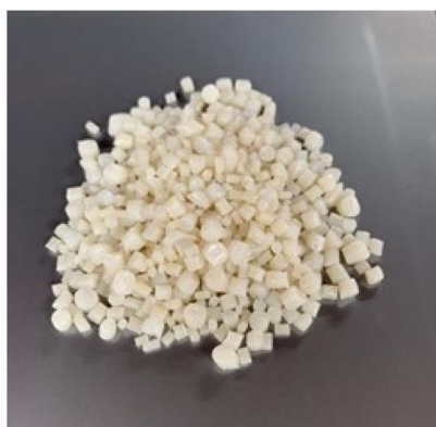
Fig. 7 Starch-based biodegradable plastic prepared with twin-axis extruder composed of 100% biomass. 54
