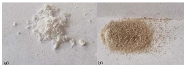
Fig. 9 Samples of precipitated glycans from (a) cold water and (b) hot water extraction.
