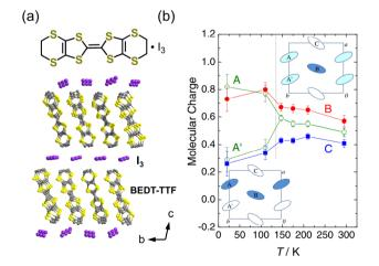
Fig. 7 (a) Crystal structure of  $\alpha$ -(BEDT-TTF)<sub>2</sub>I<sub>3</sub> (BEDT-TTF = bis(e-thylenedithio)-tetrathiafulvalene). (b) Temperature dependence of the molecular charge.<sup>43</sup> Reproduced with permission from ref. 43, The Physical Society of Japan.
