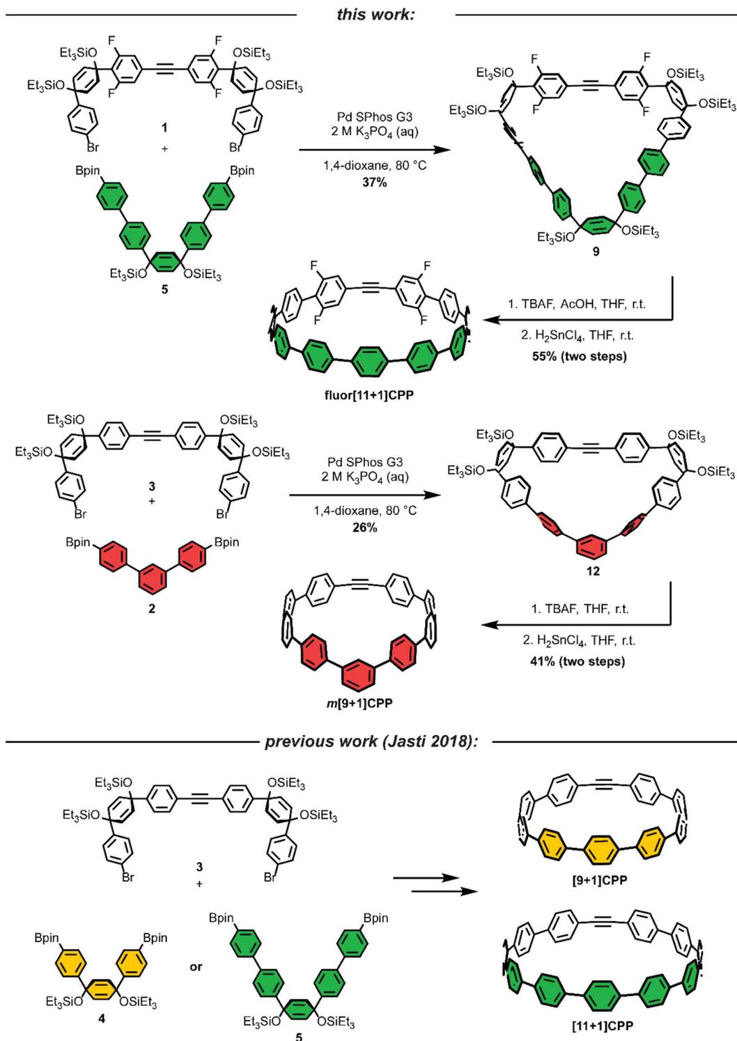
**Scheme 2** Synthesis of the  $[n+1]$ CPPs analyzed in this study. Note that the synthesis of  $[9+1]$ CPP and  $[11+1]$ CPP was first detailed in 2018 and shown here for completeness. The colors denote three important coupling partners central to this synthesis; green represents the coupling which would impart the least strain to the overall structure, while the red coupling partner would impart the most strain.
