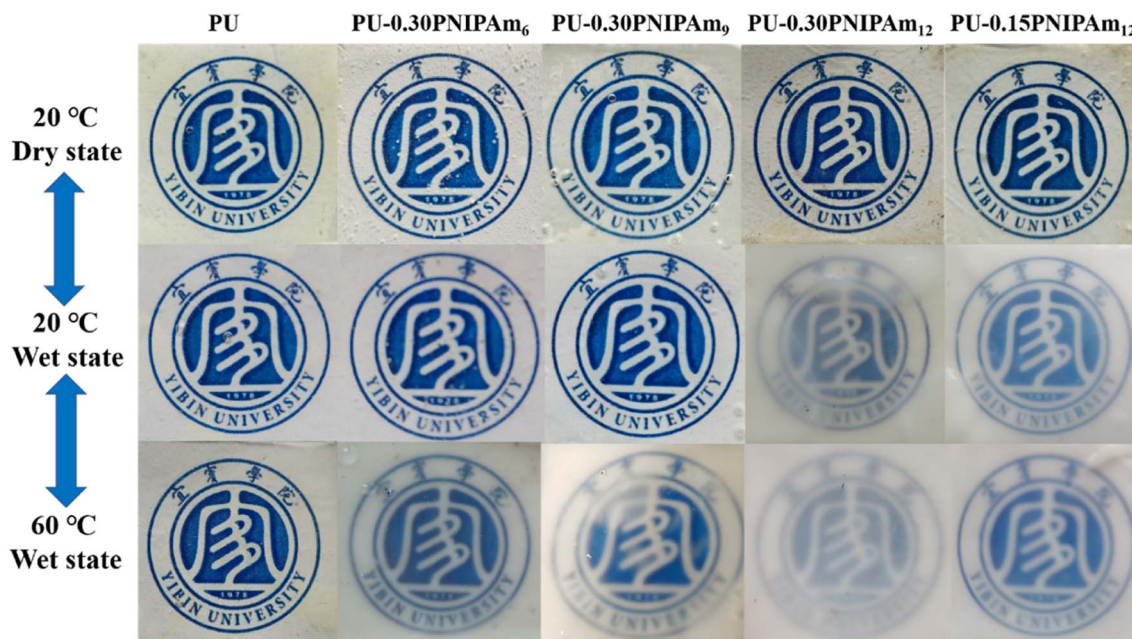
Fig. 9 The digital photographs of all samples at 20 °C (dry state, top), 20 °C (wet state, middle) and 60 °C (wet state, bottom).
