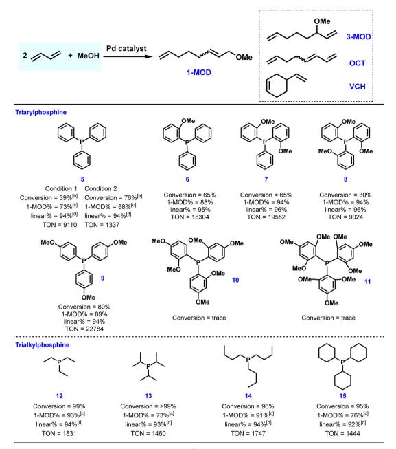
[a] condition 1: 1,3-butadiene/Pd = 32000, ligand/Pd = 2, 90 °C, 2 h; [b] in terms of 1,3-butadiene; [c] 1-MOD to the mixture of 1-MOD,3-MOD, OCT, VCH; [d] 1-MOD/(1-MOD+3-MOD); [e] condition 2: 1,3-butadiene/Pd = 2000, ligand/Pd = 2, 60 °C, 0.5 h.
