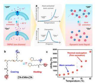
Fig. 7 (a) Design concept of a TRPV1-like heat-activated dynamic ionic liquid; (b) the reversible conversion of the dynamic ionic liquid between the polymerized state and the monomorphic state; (c) the electrical response of [TA-EMIm]TA at different temperatures. Reproduced with permission from ref. 11, copyright 2022, American Chemical Society.
