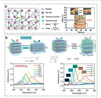
Fig. 8 (a) Photonic ionic skin embedded with silica microspheres, and the electrical/optical responsive behavior. Reproduced with permission from ref. 49, copyright 2021, Wiley-VCH. (b) Photonic hydrogel structure based on a two-dimensional bilayer membrane and the mechanisms of optical changes by external stimulation. Reproduced with permission from ref. 47, copyright 2021, American Chemical Society.
