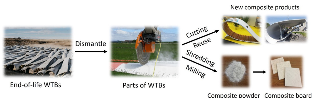
Fig. 4 Mechanical recycling processes of end-of-life WTBs.
