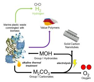
Fig. 3 Schematic showcasing the proposed theoretical tandem thermoelectrochemical (elecATT) method of producing value added products and high purity hydrogen from marine plastics commingled with biomass
