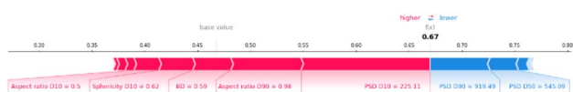
Fig. 16 SHAP force plot of the prediction of the cohesive material from the external validation that was classified as free-flowing by step 1. The red bars of the plot show the drivers that are pushing the classification toward free-flowing and the blue bars show the drivers that are pushing the classification towards non-free flowing.
