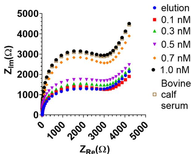
Fig. 5 EIS Nyquist plot of BHB MIP-modified BT-Au SPE electrode post-elution and after the addition of increasing concentrations of BHB (0.1 to 1.0 nM).  $\square$  refers to determination of BHB (1 nM) spiked in 1/10 diluted bovine calf serum demonstrating  $98.3\% \pm 1.5\%$  recovery.
