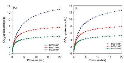
CO<sub>2</sub> uptake isotherms of carbons directly compactivated from sawdust (SD) at 600, 700 or 800 °C, and PO/SD ratio of 2 (A) or 4 (B).
