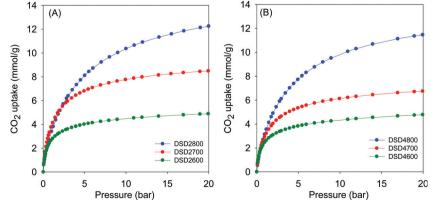
CO<sub>2</sub> uptake isotherms of carbons directly activated from sawdust (SD) at 600, 700 or 800 °C, and PO/SD ratio of 2 (A) or 4 (B).
