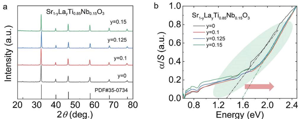
Fig. 5 Structural characterization of  $\text{Sr}_{1-y}\text{La}_y\text{Ti}_{0.85}\text{Nb}_{0.15}\text{O}_3$  ( $y = 0-0.15$ ): (a) XRD patterns and (b) absorption coefficient from the Kubelka–Munk method.
