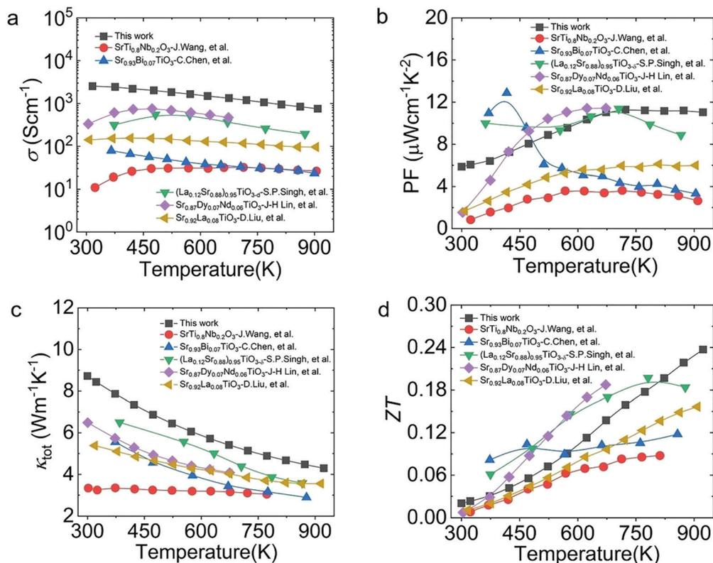
Fig. 11 Thermoelectric properties from this work and from other SrTiO<sub>3</sub>-based materials: (a)  $\sigma$ ; (b) PF; (c)  $\kappa_{\text{tot}}$ ; (d)  $ZT$ .<sup>31,42–45</sup>
