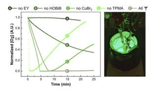
Fig. 5 Oxygen concentration measurements. Reactions conditions:  $[HOBiB]/[EYH_2]/[CuBr_2]/[TPMA] = 1/0.01/0.2/0.6$ , [HOBiB] = 1.5 mM, in PBS with DMSO (10% v/v), irradiated for 30 min under green LEDs (520 nm, 9.0 mW cm<sup>-2</sup>) in an open vial with stirring at 500 rpm.
