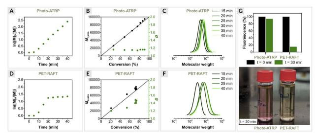
Fig. 3 Polymerization kinetics of OEOMA<sub>500</sub>, (A–C) EY/Cu mediated photo-ATRP and (D–F) EY-catalyzed PET-RAFT polymerization. (G) EY fluorescence intensity measurements.
