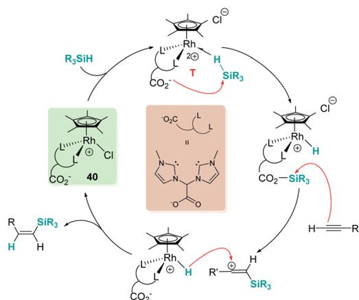
Scheme 41 Mechanism for the hydrosilylation of alkynes by **40**.
