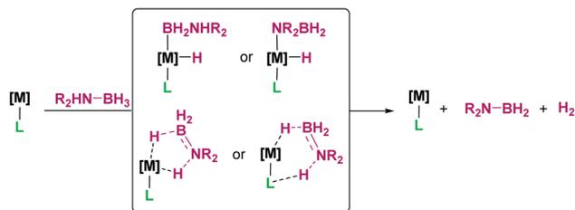
Scheme 58 Classical mechanisms for metal-catalysed dehydrocoupling of amine-boranes.
