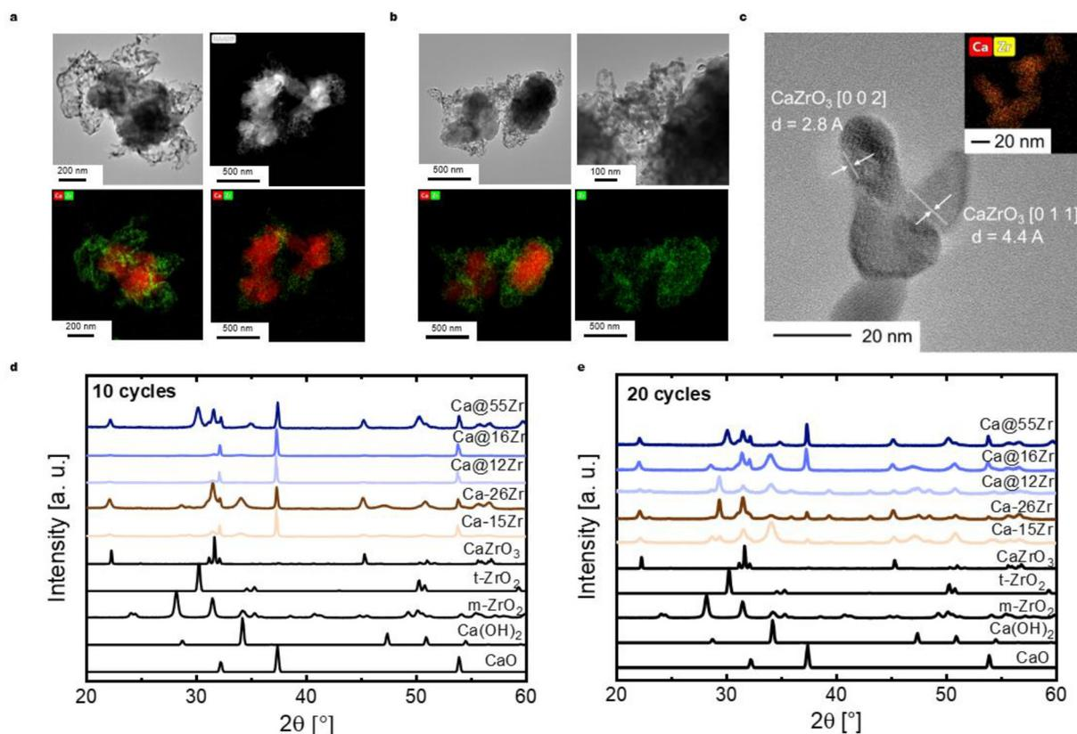
**Fig. 5** (a) (EDX)-TEM analysis of the most effective yolk-shell-structured sorbent Ca@12Zr after 10 carbonation–calcination cycles, (b) (EDX)-TEM analysis of the core-shell-structured sorbent Ca-26Zr, (c) high-resolution TEM micrograph and EDX mapping of the dendritic structures observed for all zirconia-stabilized sorbents (here: Ca@16Zr) and XRD patterns of the zirconia-stabilized sorbents after (d) 10 carbonation–calcination cycles as well as (e) 20 carbonation–calcination cycles.
