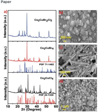
Fig. 3 (a) X-ray diffraction pattern of Cs<sub>2</sub>CuCl<sub>4</sub>, Cs<sub>2</sub>CuBr<sub>4</sub> and Cs<sub>2</sub>CuBr<sub>2</sub>Cl<sub>2</sub>. (b-d) SEM images of Cs<sub>2</sub>CuCl<sub>4</sub>, Cs<sub>2</sub>CuBr<sub>4</sub> and Cs<sub>2</sub>CuBr<sub>2</sub>Cl<sub>2</sub> present square shaped nanoplates, nanorods and rectangular shaped nanoplates, respectively.
