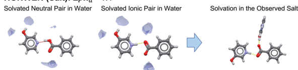
Fig. 10 Visualisation of water solvation of non-ionised versus ionised acid–base pairs with full interaction maps versus the resulting ionisation and interactions observed in their crystals.
