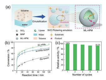
Fig. 4 (a) Schematic illustration of interfacial catalysis in the water-intoluene Pickering emulsions stabilized by 1% ML-HPMs. (b) Conversion of 1-hexanol and hexanoic acid to ester with the reaction time for free lipase in a water-toluene biphasic system; free lipase was in the water phase of the w/o Pickering emulsion stabilized by M-HPMs and the w/o Pickering emulsion stabilized by ML-HPMs. (c) Reusability of ML-HPMs for 5 cycles.
