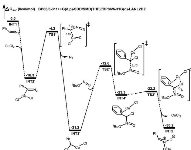
Fig. 2 Energy profile (in  $\text{kcal mol}^{-1}$ ) for the formation of nitronate with the  $\text{CuCl}_2$  catalyst. Bond lengths are shown in Å.
