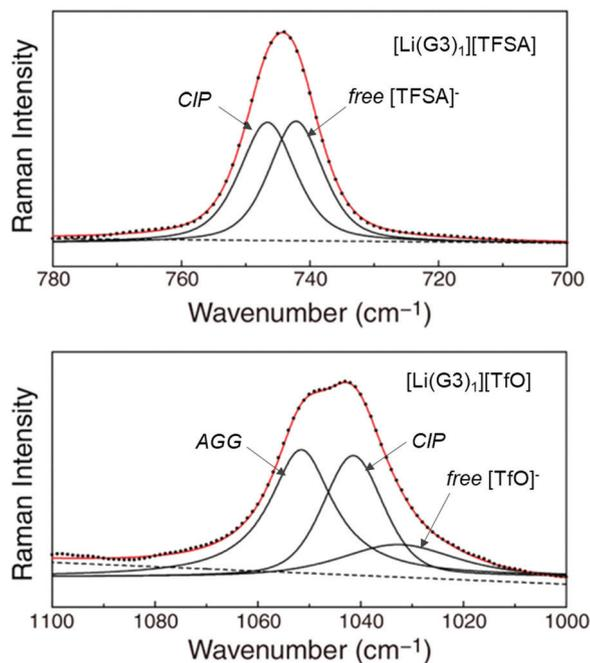
Fig. 6 Raman spectra of  $[\text{Li}(\text{G3})_1][\text{TFSA}]$  in the range  $700\text{--}780\text{ cm}^{-1}$  (top,  $\text{CF}_3$  bending mode) and of  $[\text{Li}(\text{G3})_1][\text{TfO}]$  in the range  $1000\text{--}1100\text{ cm}^{-1}$  (bottom,  $\text{SO}_3$  stretching mode) at  $60\text{ }^\circ\text{C}$ . Reprinted with permission from ref. 58 Copyright 2014 American Chemical Society.
