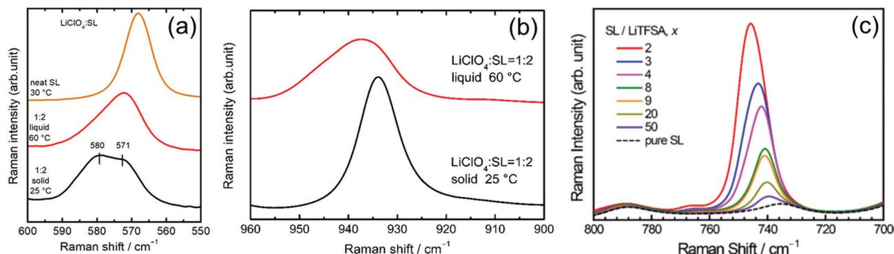
Fig. 9 Raman spectra of (a) scissoring mode of the  $\text{SO}_2$  group of SL and (b) Cl–O symmetric stretch vibration mode of  $\text{ClO}_4^-$  in the  $[\text{Li}(\text{SL})_2][\text{ClO}_4]$  solvate. Reprinted with permission from ref. 31 Copyright 2018 American Chemical Society. (c) Raman spectra of the S–N stretching vibration mode of  $\text{TfSA}^-$  anion in the LiTfSA/SL binary mixtures. Reprinted with permission from ref. 39 Copyright 2019 American Chemical Society.
