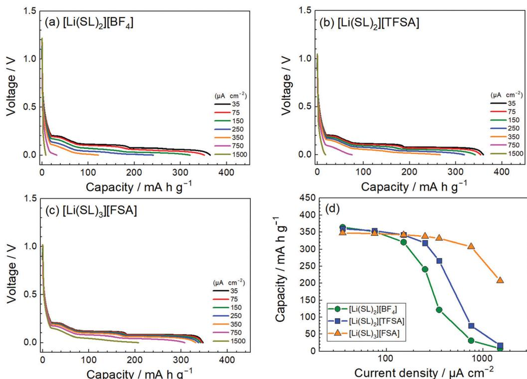
Fig. 14 Charge curves for the Li/graphite cells containing electrolytes of (a) [Li(SL)<sub>2</sub>][BF<sub>4</sub>], (b) [Li(SL)<sub>2</sub>][TFSA], and (c) [Li(SL)<sub>3</sub>][FSA] at various current densities at 30 °C. (d) Charge capacities of the cells as functions of current density. Following each charge measurement, the cell was fully discharged at the low current density of 35  $\mu\text{A cm}^{-2}$ .
