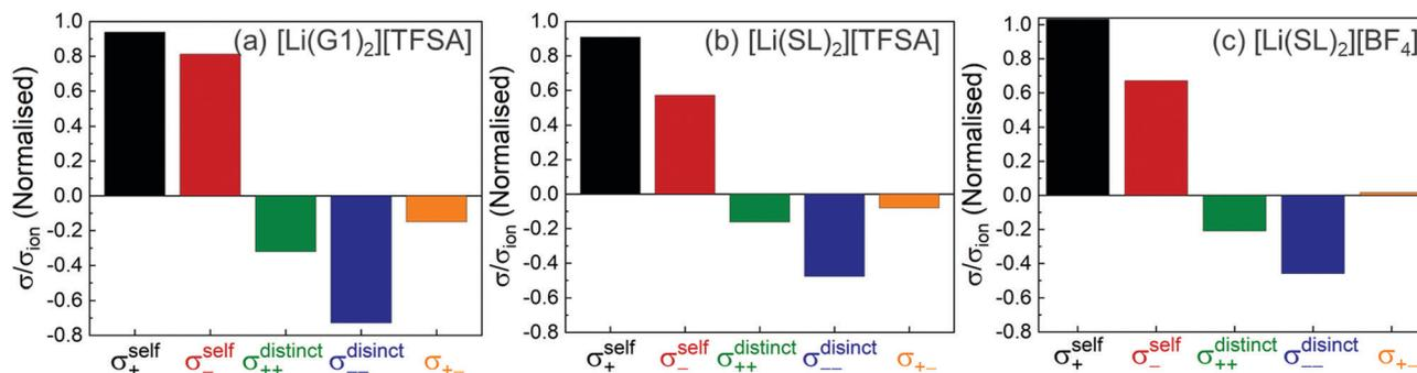
Fig. 12 Normalised Onsager transport coefficients ( $\sigma_{+}^{self}/\sigma_{ion}$ ,  $\sigma_{-}^{self}/\sigma_{ion}$ ,  $\sigma_{++}^{distinct}/\sigma_{ion}$ ,  $\sigma_{--}^{distinct}/\sigma_{ion}$ , and  $\sigma_{+-}/\sigma_{ion}$ : left to right) of (a) [Li(G1)<sub>2</sub>][TFSA], (b) [Li(SL)<sub>2</sub>][TFSA], and (c) [Li(SL)<sub>2</sub>][BF<sub>4</sub>]. The graphs (a) and (b) are reprinted with permission from ref. 87. Copyright 2020 PCCP Owner Societies.
