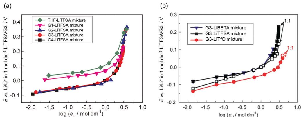
Fig. 3 Plots of the  $\text{Li}/\text{Li}^+$  electrode potential against a common logarithm of the Li salt concentration in (a) G4 (tetraglyme), G3 (triglyme), G2 (diglyme), G1 (monoglyme), and THF–LiTfSA mixtures; (b) G3–LiTfO, –LiTfSA, and –LiBETA mixtures at 30 °C. Reference electrode was  $\text{Li}/\text{Li}^+$  in 1 mol  $\text{dm}^{-3}$  LiTfSA/G3. (b) was reprinted with permission from ref. 59 Copyright 2015 PCCP Owner Societies.
