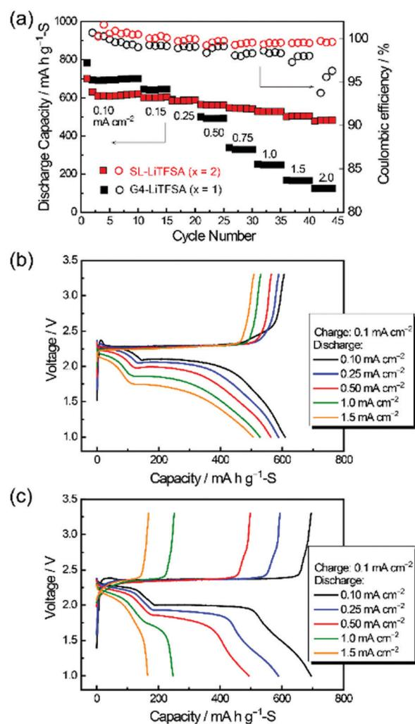
Fig. 18 (a) Discharge capacity and Coulombic efficiency at different discharge current densities, and charge and discharge curves of the cells using the concentrated electrolytes, (b)  $[\text{Li}(\text{SL})_2][\text{TfSA}]$  and (c)  $[\text{Li}(\text{G4})_2][\text{TfSA}]$ . Reprinted with permission from ref. 39 Copyright 2019 American Chemical Society.
