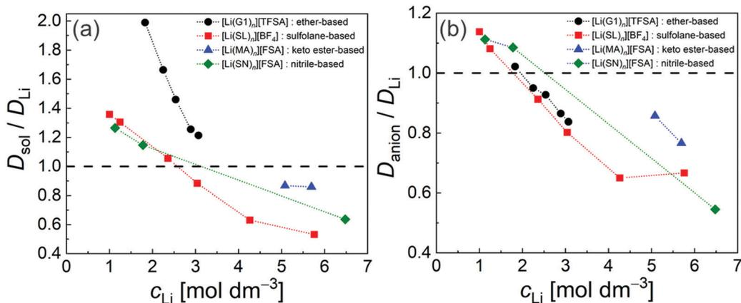
Fig. 10 Diffusivity ratio (a)  $D_{\text{sol}}/D_{\text{Li}}$  and (b)  $D_{\text{anion}}/D_{\text{Li}}$  of ether-, sulfonate-, keto ester-, and nitrile-based electrolytes at 30 °C. ([Li(G1) $_n$ ][TFSA]:  $n = 1.8, 2, 2.5, 3,$  and  $4$ ; [Li(SL) $_n$ ][BF $_4$ ]:  $n = 1.35, 2, 3, 4, 8,$  and  $10$ ; [Li(MA) $_n$ ][FSA]:  $n = 0.8$  and  $1$ ; and [Li(SN) $_n$ ][FSA]:  $n = 0.8, 6$  and  $10$ ). Data were collected from ref. 31, 61, 72 and 73 and replotted.
