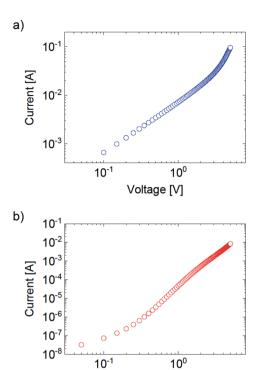
Fig. 6 Space-charge limited current (SCLC) vs. voltage curves for the 300 nm-thick PM6:Y6 devices with the following structures: (a) ITO/ ZnO/PM6:Y6/PDINO/Aq, (b) ITO/PEDOT:PSS/PM6:Y6/MoO<sub>3</sub>/Au
