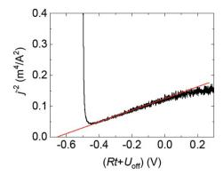
Fig. 4 Experimental current density transient obtained in the CELIV measurement for the 300 nm thick PM6:Y6 device at the pulse rampup rate of 0.8 V/50  $\mu$ s and the offset voltage of -0.5 V
