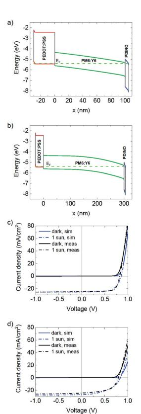
Fig. 5 Simulated energy band diagrams at the "short circuit" condition (a and b) and comparison of simulated and measured J-V characteristics (c and d) of the PM6:Y6 devices with active layer thicknesses of 100 nm (a and c) and 300 nm (b and d). See Table 1 for simulation parameter details.
