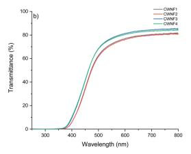
Fig. 4 UV and visible light (a) absorption coefficient and (b) transmittance of CWNF films, showing strong absorption behavior in the UV region (<400 nm) and high transparency in the visible light region (380-760 nm (ref. 61)).
