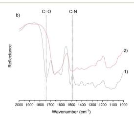
Fig. 1 (a) the DRIFT spectra of wood (1) and cationic wood obtained using urea as carbamide (2), and (b) the fingerprint region of the DRIFT spectra showing the most distinguished differences between the two spectra: the disappearance of the carbonyl peak (C=O) of the ester bond and the appearance of a carbon-nitrogen peak (C-N) after chemical modification.
