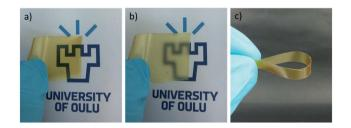
Fig. 3 CWNF film (a) directly on top and (b) held a few centimeters above the background showing good transparence and a slight haziness of the films, and (c) bending of the film to demonstrate good mechanical robustness.
