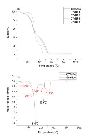
Fig. 6 (a) TGA curves of original sawdust and CWNF films and (b) DTG curve of the CWNF4 film with original sawdust.
