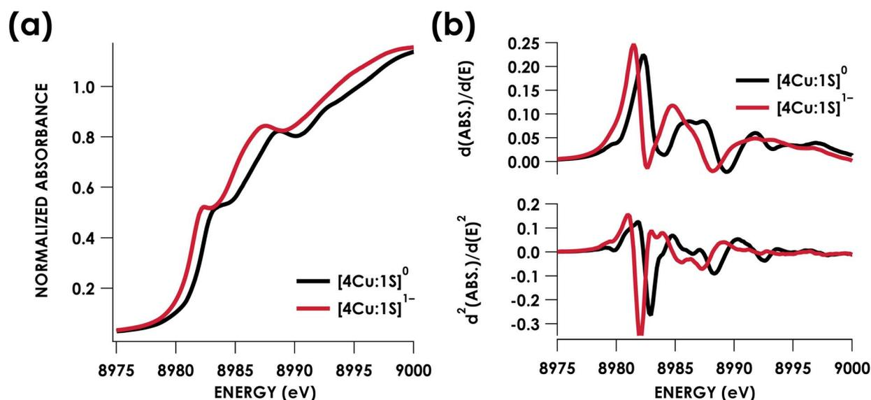
Fig. 3 (a) Cu K-edge XAS spectra obtained for the  $[4\text{Cu}:1\text{S}]^{0/1-}$  redox couple. (b) First (top) and second (bottom) derivative Cu K-edge XAS spectra. Isoenergetic pre-edge ( $1s \rightarrow 3d$ ) excitations are evident in the second-derivative spectra at 8979.8 eV. Rising edge inflection points occur at 8982.3 and 8985.9 eV for  $[4\text{Cu}:1\text{S}]^0$  and 8981.5 and 8984.8 eV for  $[4\text{Cu}:1\text{S}]^{1-}$ .
