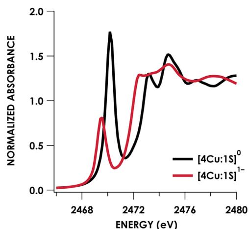
Fig. 4 S K-edge XAS data obtained for the  $[4\text{Cu}:1\text{S}]^{0/1-}$  redox couple. Pre-edge peaks corresponding to  $\text{S } 1s \rightarrow \psi^*$  excitations are located at 2470.2 eV for  $[4\text{Cu}:1\text{S}]^0$  and 2469.5 eV for  $[4\text{Cu}:1\text{S}]^{1-}$ .
