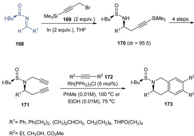
Scheme 29 The synthetic route to 3,6,7-trisubstituted 1,2,3,4-tetrahydroquinolines.
