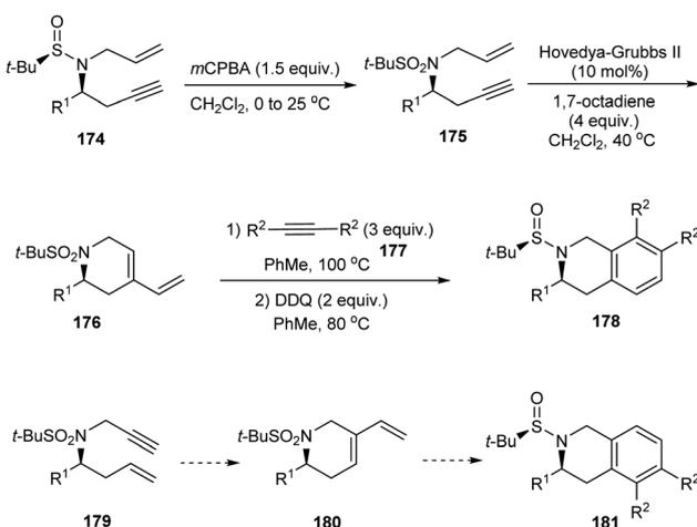
Scheme 30 The synthetic route to 7,8-disubstituted 1,2,3,4-tetrahydroquinolines.
