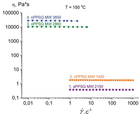
Fig. 33 Dependence of viscosity on the shear rate (flow curves) at 150 °C for the PPSQ obtained.<sup>25</sup> Reproduced with the permission of Elsevier publishing.
