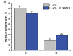
Fig. 12 (a) Carbon hybridization fractions and (b) relative concentrations of carbon and hydrogen in a-C before and after exposure to H radicals.
