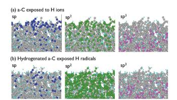
Fig. 11 Side view of the a-C model: (a) exposed to 50 eV H ions at the fluence of  $8\times10^{15}\,\mathrm{cm^{-2}}$ , and (b) exposed to H ions and H radicals at 300 K and the fluence of  $10^{17}\,\mathrm{cm^{-2}}$ .
