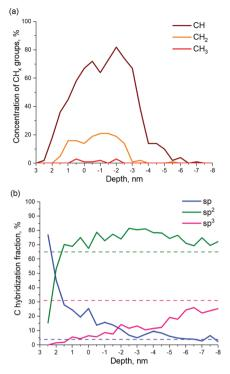
Fig. 10 (a) Relative concentration of CH<sub>x</sub> groups in the H-modified a-C and (b) calculated profiles of carbon hybridization in the H-modified a-C layer. The initial values of sp, sp<sup>2</sup> and sp<sup>3</sup> hybridization are shown by dashed lines of the corresponding color.
