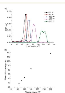
Fig. 7 (a) Ion energy distribution function for various plasma power settings obtained in PIC MCC simulation. (b) Mean H ion energy as the function of the plasma power.
