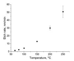
Fig. 2 H radicals based etch rate of a-C as a function of substrate process temperature.
