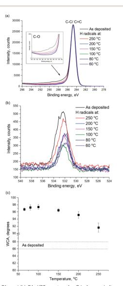
Fig. 3 (a) C1s and (b) O1s XPS spectra of a-C before and after remote H plasma treatment at various temperatures, (c) WCA of a-C before and after remote H plasma treatment at various temperatures.
