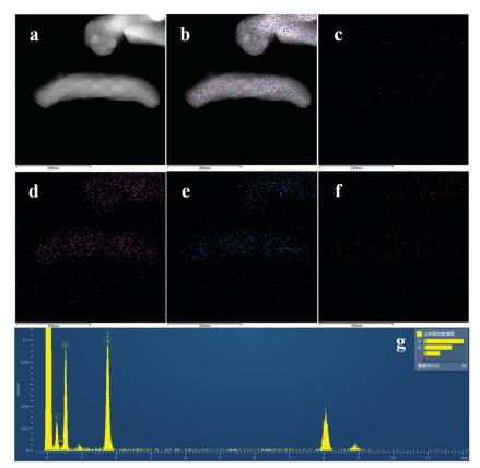
Fig. 4 TEM images of MSNR2 (a and b), elemental mapping of N (c), Si (d), O (e) and C (f), respectively, and EDAX result (g).
