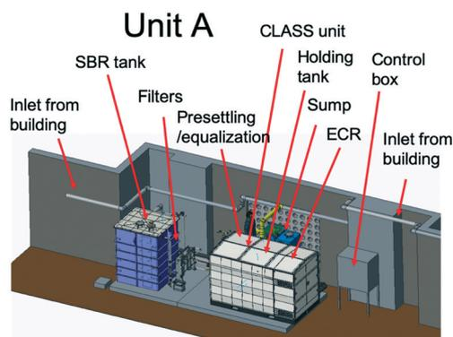
**Fig. 2** Layout of the installation at site A with a SBR biological pre-treatment system.
