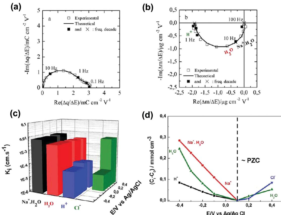
Fig. 8 (a) and (b) The transfer functions  $\frac{\Delta q}{\Delta E}(\omega)$  and  $\frac{\Delta m}{\Delta E}(\omega)$  at  $-0.4$  V vs. Ag/AgCl, respectively. (c) The kinetic parameters  $K_i$  ( $\text{cm s}^{-1}$ ) for each ion at different applied potentials. (d) Relative concentration variation of each ion in SWCNT based thin films as a function of potential in  $0.5$  M NaCl at  $\text{pH} = 7$ . Reproduced from ref. 173 with permission from Elsevier (copyright 2016).
