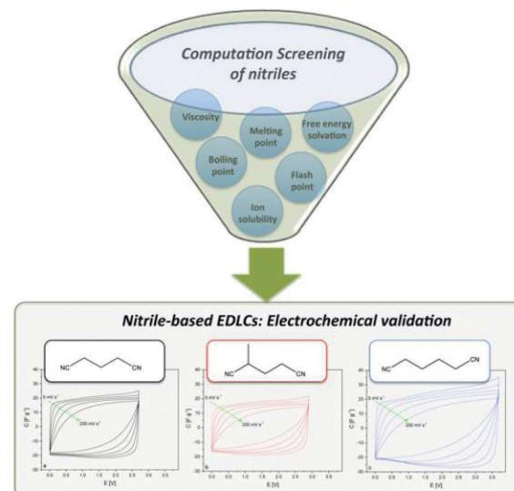
Fig. 15 (a) The screening strategy based on computational methods. (b) An illustration abstract for selecting a new solvent for supercapacitor applications. The figure is reproduced from ref. 336 with permission from 2008 American Chemical Society.
