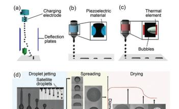
Fig. 5 Inkjet printing principles: schematics of (a) CIJ, and DOD inkjet printing with (b) piezoelectric and (c) thermal head; (d) the complete inkjet printing process, showing the droplet jetting, spreading and drying stages. Reproduced with permission from ref. 98. Copyright 2018, Royal Society of Chemistry.
