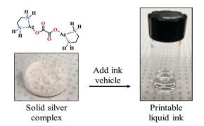
Fig. 18 Solid silver complex that can be converted to a desired printable liquid ink. Reproduced with permission from ref. 99. Copyright 2018, American Chemical Society
