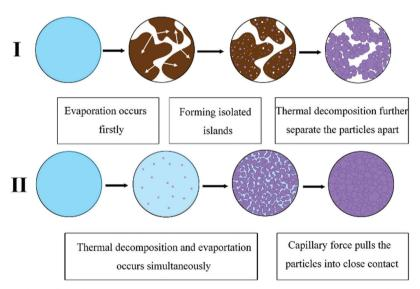
Fig. 20 Schematic presentation of the effect of amines on microstructure evolution. Reproduced with permission from ref. 75. Copyright 2016 Elsevier.
