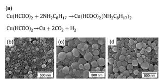
Fig. 21 (a) Chemical reaction in the as-prepared copper formic ink during synthesis and sintering processes; (b–d) SEM images of the copper conductive film obtained by calcination for 60 min at 110  $^{\circ}$ C, 140  $^{\circ}$ C, and 160  $^{\circ}$ C. Reproduced with permission from ref. 52. Copyright 2011 Elsevier.
