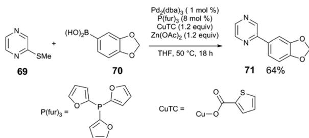
**Scheme 18** Pd-Catalyzed coupling of arylthioethers and boronic acids.<sup>84</sup>
