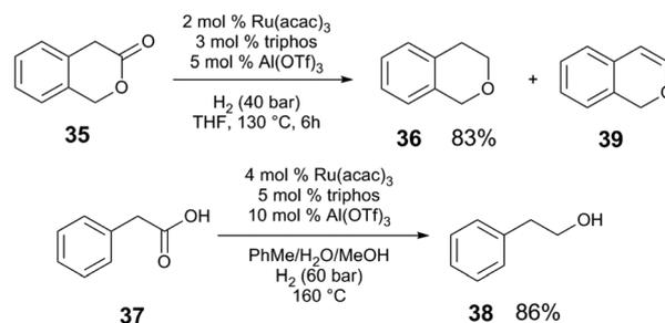
**Scheme 10** Hydrogenation of esters<sup>45</sup> (top) and carboxylic acids<sup>46</sup> (bottom).
