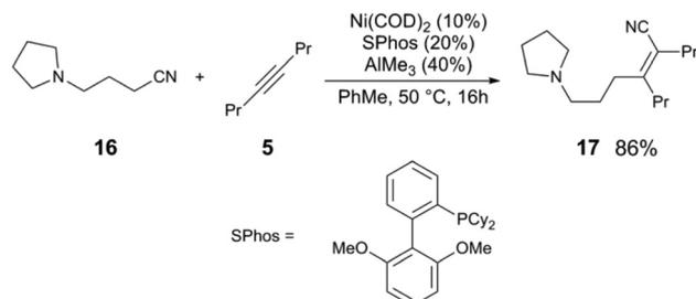
Scheme 5 Activation of alkylnitriles using a directing group.<sup>24</sup>
