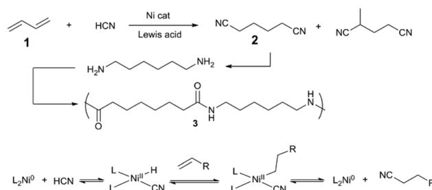
**Scheme 1** Hydrocyanation of butadiene *en route* to 6,6-nylon (**3**)<sup>6</sup> (top) and the mechanism of Ni-catalysed alkene hydrocyanation (bottom).
