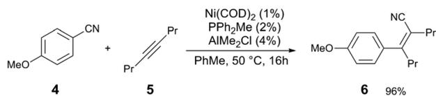
Scheme 2 Ni and Al-catalysed carbocyanation of alkyne with benzonitriles.<sup>11</sup>
