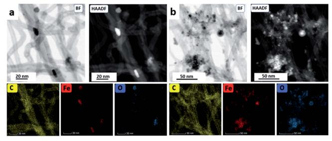
Fig. 4 (a) BF and HAADF-STEM images of  $Fe_3O_4@MWCNT$  (collected) with the corresponding STEM element mapping. (b) BF and HAADF-STEM image of  $Fe_3O_4@MWCNT$  (retained) with the corresponding STEM element mapping.
