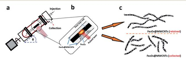
Fig. 1 Schematic illustration of the experimental procedure for the preparation for Fe<sub>3</sub>O<sub>4</sub>@MWCNT. (a) The vortex fluidic device (VFD) and laser Nd:YAG processing at 1064 nm. (b) Zoomed in schematic for generating Fe<sub>3</sub>O<sub>4</sub> NPs under laser irradiation of an iron rod (power at 250 mJ). (c) Fe<sub>3</sub>O<sub>4</sub>@MWCNT exiting the tube under continuous flow (collected) and retained in the tube.
