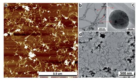
Fig. 2 (a) AFM image, (b) STEM image, (c) HRTEM image and (d) TEM of Fe<sub>3</sub>O<sub>4</sub>@MWCNT (retained), formed in the VFD (optimised parameters) operating at 8.5k rpm rotational speed, under continuous flow, with the concentration of the as received MWCNTs at 0.08 mg mL<sup>-1</sup> (DMF), tilt angle 45°, flow rate 0.45 mL min<sup>-1</sup>, and laser power 250 mJ, with the MWCNTs ca. 2 μm in length.
