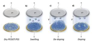
Fig. 2 Voltage induced swelling/shrinkage of PEDOT:PSS film. (a) Dry film on a gold coated EQCM-D sensor, (b) swelling when in contact with the electrolyte, (c) additional swelling during de-doping due to up-take of Na<sup>+</sup> ions and water, (d) shrinkage when the potential is reversed. We record significant differences in the volumetric expansion as well as the reversibility of the de-doping process depending on the film thickness.
