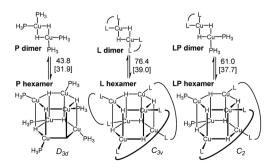
Scheme 5 Energy of the model dimers relative to the corresponding hexameric CuH aggregates. Ligands are truncated (see ESI† for details).<sup>31</sup>
