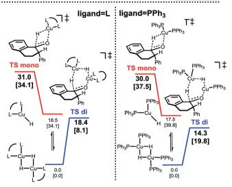
**Scheme 6** Relative energetics of monomeric (red) and dimeric (blue) hydride transfer pathways for bidentate (left) and monodentate (right) ligands.<sup>31</sup>
